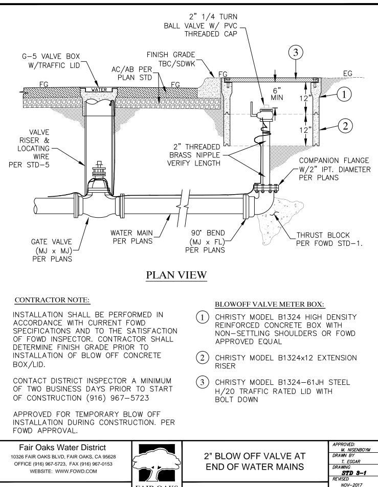
N:\AUTOCAD FILES\AUTOCAD MASTER DWGS\WORKING DWGS\Standard SPEC Dwgs\Std-Dwg FOWD\Dwgs\Std-3-1 Blowoff-End Main.dwg, 11/29/17 10:54:24am, teggar
